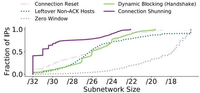
Figure 4: **Network Granularity of TCP Blocking**—Some protections appear to be host-based while others are more prevalent on large networks. Zero Window DDoS protections are most likely to appear at a large network granularity, while connection shunning is more likely a host-level behavior.
