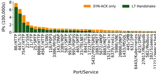
Figure 1: **L4 vs. L7 Responsiveness**—A significant fraction of hosts that respond with a SYN-ACK packet never complete the expected application-layer handshake. The difference varies dramatically across ports by both percent difference (14–96%) and raw count (21,050–200,902).
