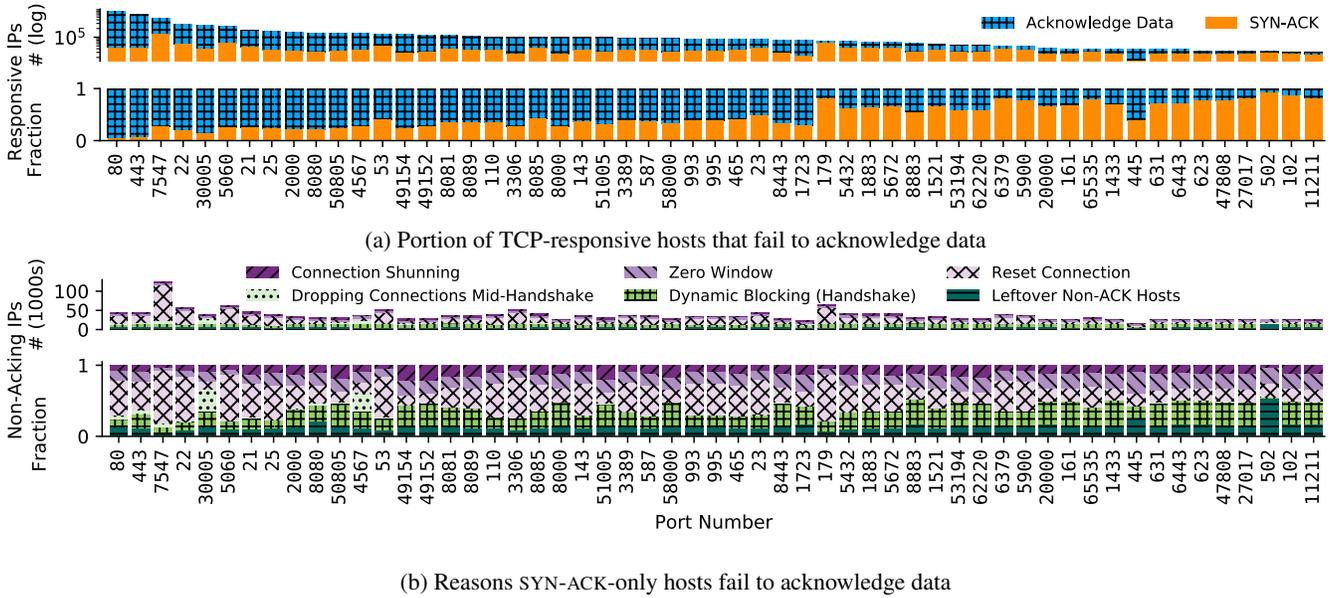
Figure 3: **Unexpected TCP Behavior of IPv4 Hosts**—An average 16% of services on popular ports and 40% of services on unpopular ports that respond to a TCP SYN scan with a SYN-ACK packet do not fully speak TCP. Here, we show the portion of hosts by port that do not acknowledge client data and the breakdown of reasons why.
