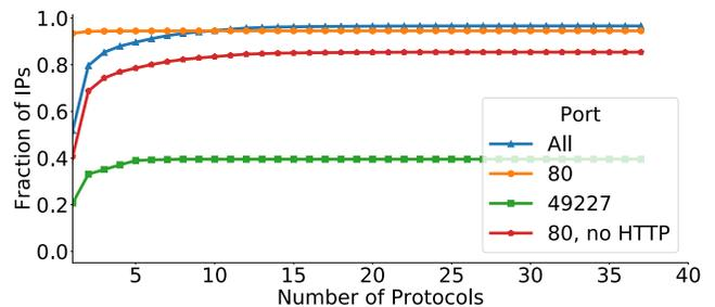
Figure 8: **Protocol Coverage Convergence**—The marginal gain of scanning additional protocols is negligible beyond the top 10 protocols. Still, for most ephemeral ports (e.g., port 49227) the majority of services remain unknown.
