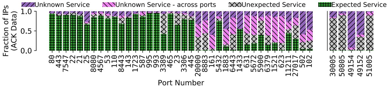
Figure 6: **Distribution of Types of Services**—A smaller fraction of services run the assigned protocol on less popular ports. For example, only 4% of services on TCP/102 speak the assigned S7 protocol. The fraction of services that can be identified on unassigned ports (on the right hand side) varies widely.
