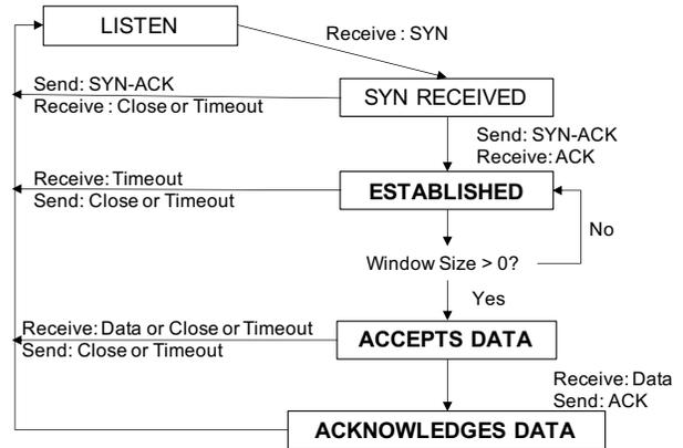
Figure 2: **Client Perspective of Server TCP State**—We investigate L7 service liveness based on a modified version of the TCP state machine in RFC 793 [54]. We introduce two new states: “accepts data” and “acknowledges data” because an established connection cannot necessarily exchange data.
