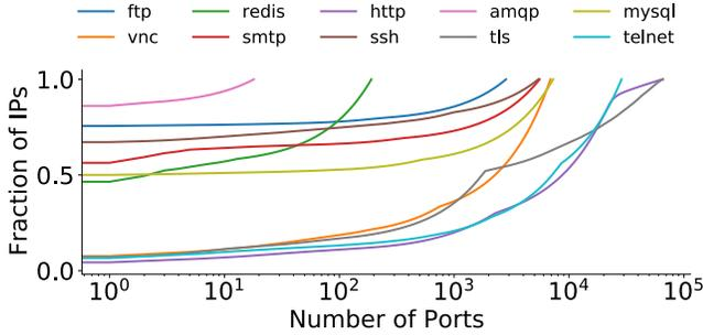
Figure 9: **Protocol Coverage Across Ports**—Only 3.0% of HTTP services are served on port 80. Researchers must scan 25K ports to achieve 90% coverage of HTTP services. On the other hand, 83.1% of AMQP services are on port 5672.
