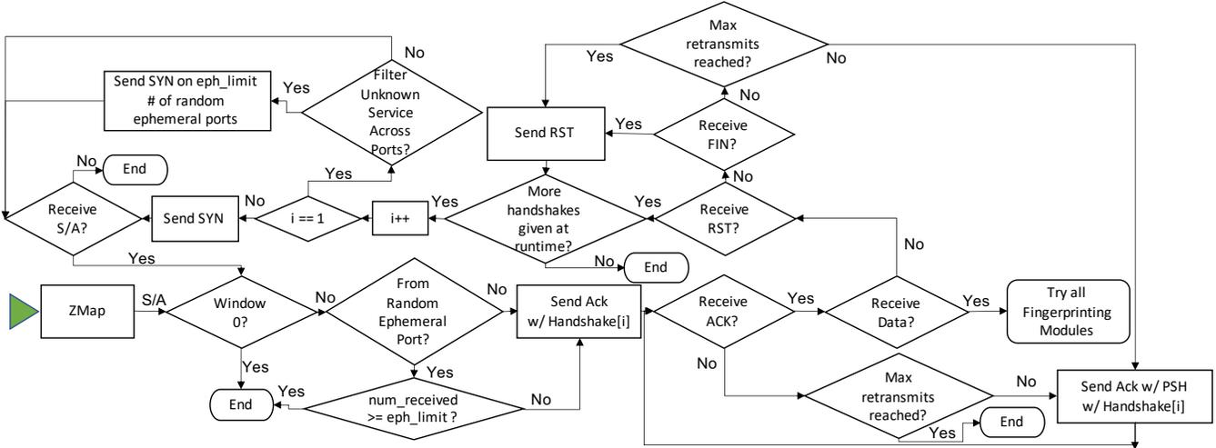
Figure 12: **LZR Algorithm**—LZR efficiently identifies real Internet services by sending application-layer data with the ACK of a TCP handshake to filter out non-acknowledging hosts and fingerprint the responding protocol.
